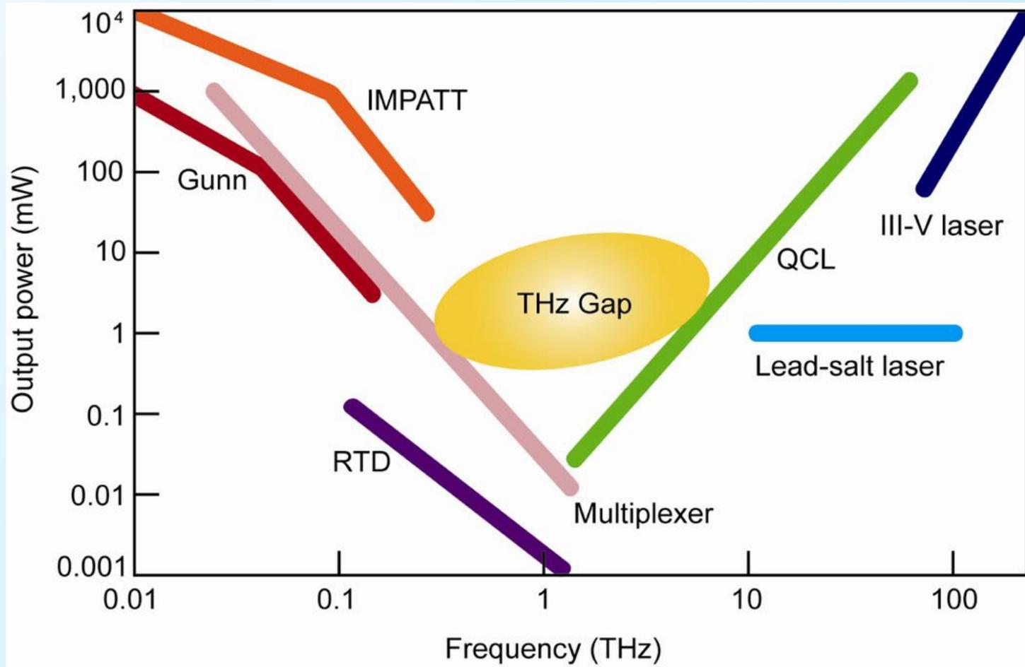
RTD: Resonant tunnel diode; IMPATT: Impact ionization avalanche transit-time diode; QCL: Quantum-cascade laser.
